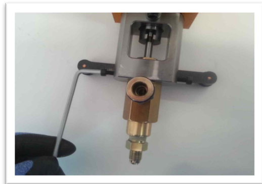
7. Assemble : Screw the two bolts tightly.
