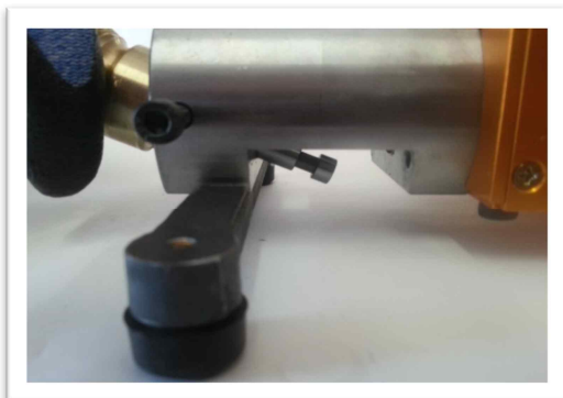
3. Disassemble : Separate the old damaged piston downwards.
