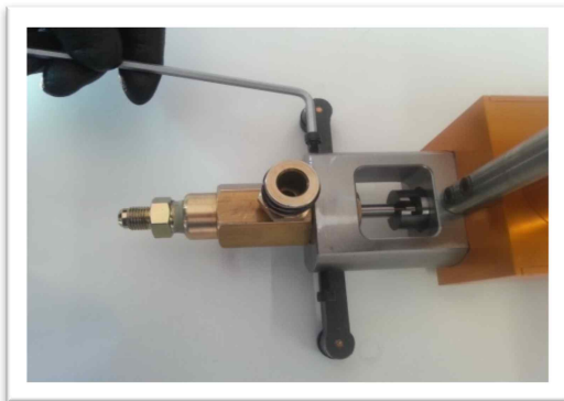
1. Disassemble : Unscrew the two bolts by using wrench.
