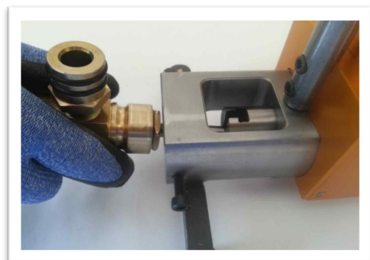
5. Assemble : Insert new piston, and fix into the rod-shaft's groove to up from below, as the picture.
