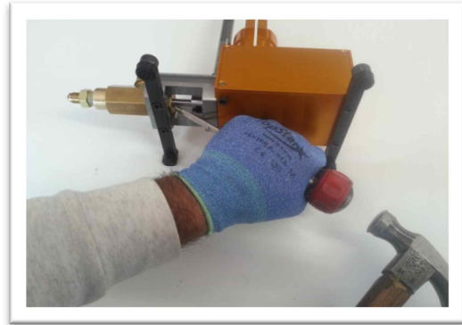
4. Disassemble : In case the damaged piston doesn't separate from joiner, please, use chisel and hammer in order to separate as the picture.
